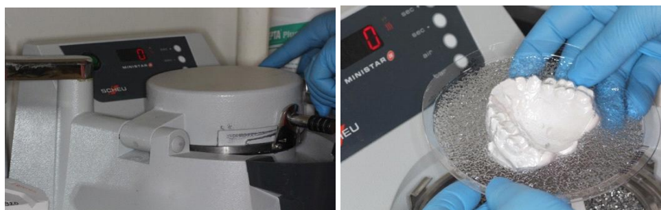
Fig. 9. Obtaining the aligner after reaching the optimum parameters and after the thermo vacuum forming process
