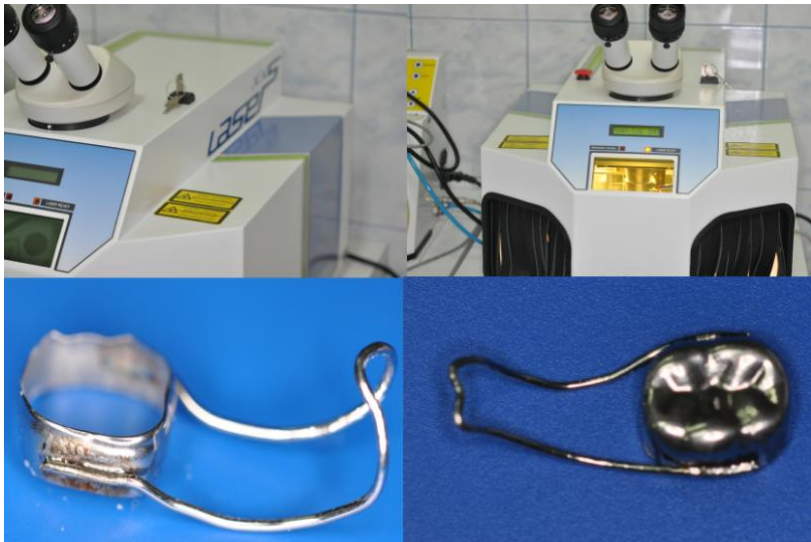
Fig. 9.8 Laser welding of the space maintainer (Collection of the Department of Pediatric Dentistry)
